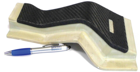
3D printed motorcycle rear fender support
